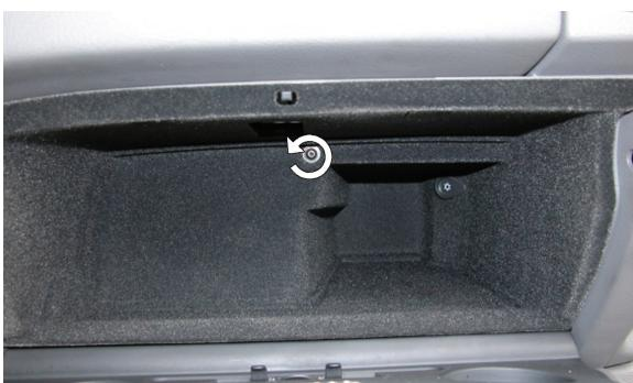
(EN) Loosen the screw and remove housing
