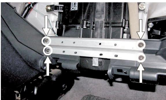
**EN** Remove the protecting device
