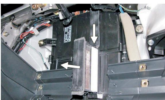
Carefully remove the first filter, the second one will slide downwards. Carefully remove the second filter, install the new one and perform the previous actions in the opposite order
