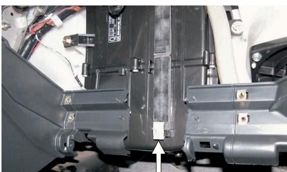
**EN** Remove the filter fastener
