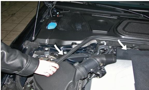
(EN) Remove the rubber seal
