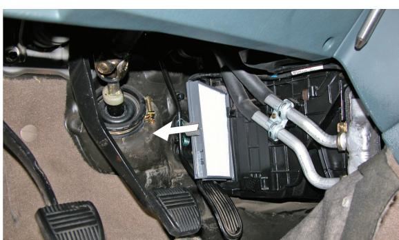
Carefully remove the first filter, the second one will slide downwards. Carefully
