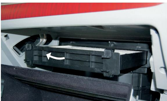
(EN) Remove the old filter, insert the new one and carry out the opposite to all the previous operation in the reversed order
