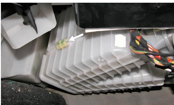
(EN) Open the locks which hold the filter housing
