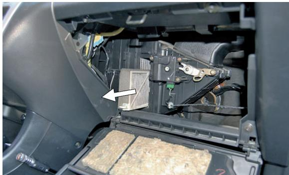
**(EN)** Carefully remove the old filters, put in the new ones and perform the opposite to all the previous steps in the reversed order
