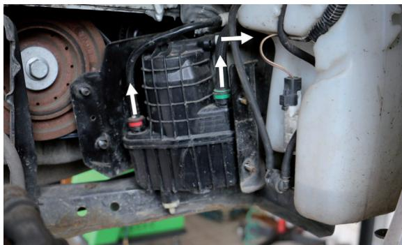
(EN) Disconnect the quick connects of fuel filter pipes
