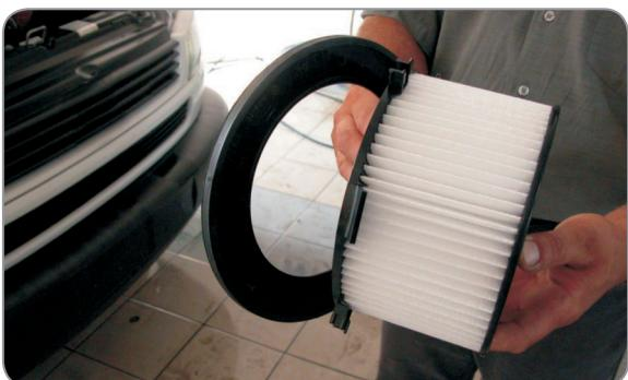
**(EN)** Detach the cover of the filter cartridge, insert the replacement and perform the previous actions in the opposite order
