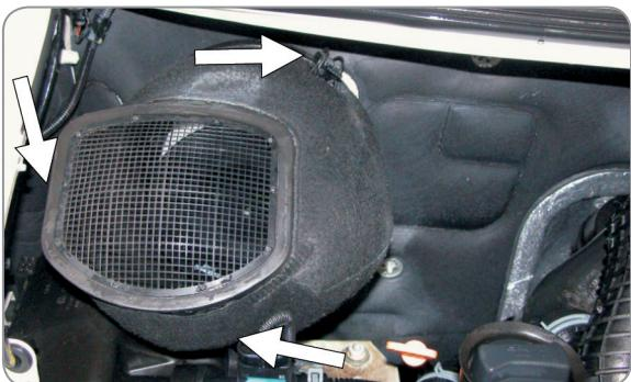
**(EN)** Unfasten the dips of filter cartridge housing
