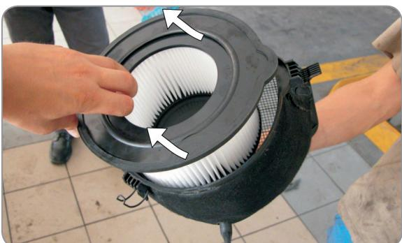
**(EN)** Detach the cover of the filter cartridge
