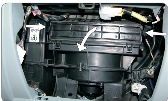
EN Unlatch the filter with the frame from its socket
