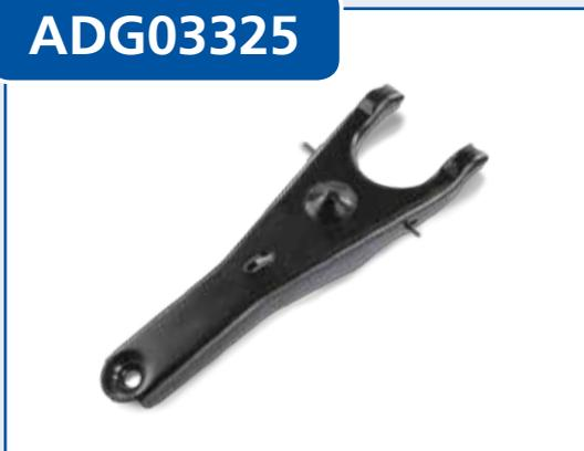
We have found that the cause of the problem can lie with a crack in the clutch release fork, as the release fork on this model can fracture and flex during operation and not allow the clutch to fully disengage.
