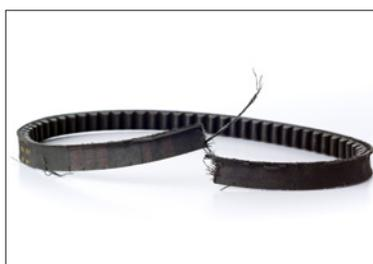
**Cause: Failure of belt tensioner J1140337 on account of inexpert installation**
